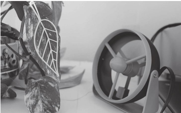
A fan blowing air onto a leaf with a prototype attached to it, to demonstrate how energy can be captured from the leaf’s movement.
